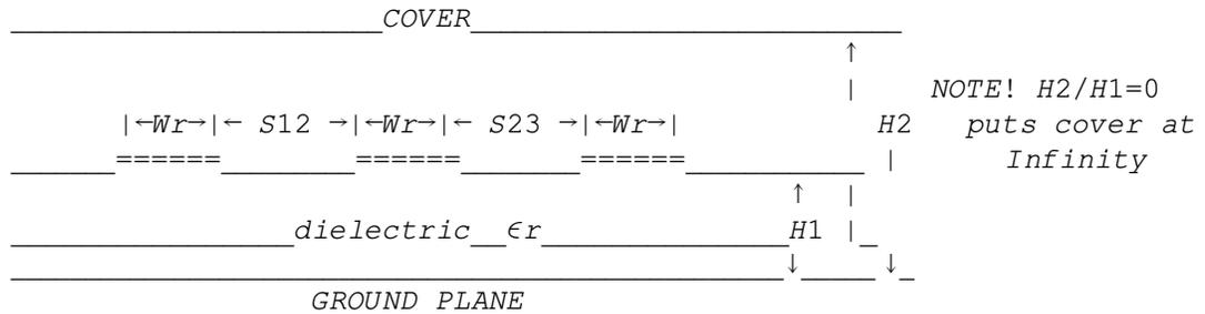
Figure 6.2. Cross-section of combline filter substrate & cover
