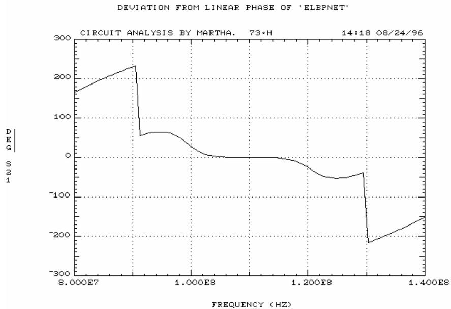
Figure 8.5. Deviation from linear phase of elliptic filter
