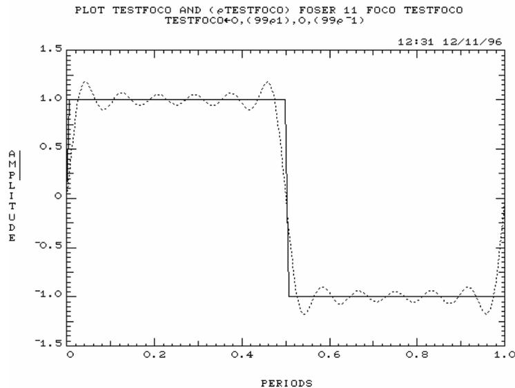
Figure 10.7. Fourier series decomposition of a square wave up to 11<sup>th</sup> harmonic
