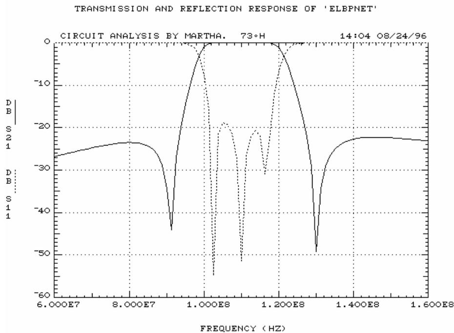
Figure 8.1. Frequency response of 3rd order elliptic filter
