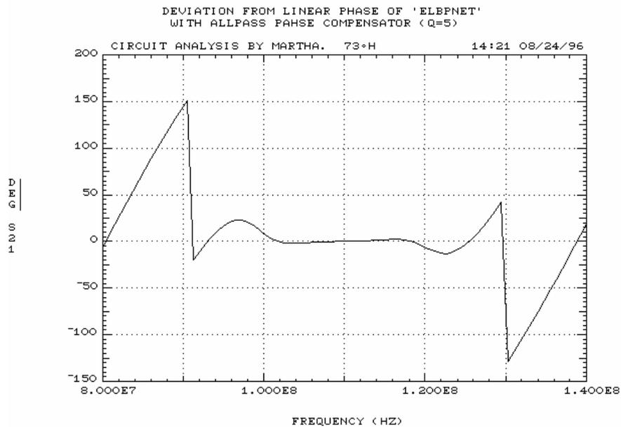
Figure 8.6. Elliptic filter with all-pass phase compensator
