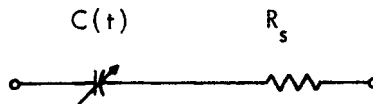
Figure 22. Varactor diode model, the capacitance C(t) has components at the pump frequency f_p and at 2f_p .
